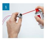
Remove rough dirt like dust from **connector and receptacle** by using compressed air.
