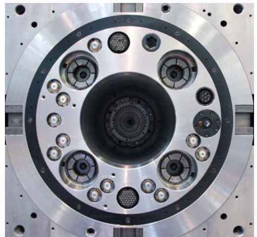
ODU DOCK FOR MILLING AND GRINDING MACHINES (Source: Waldrich Siegen Werkzeugmaschinen GmbH)
